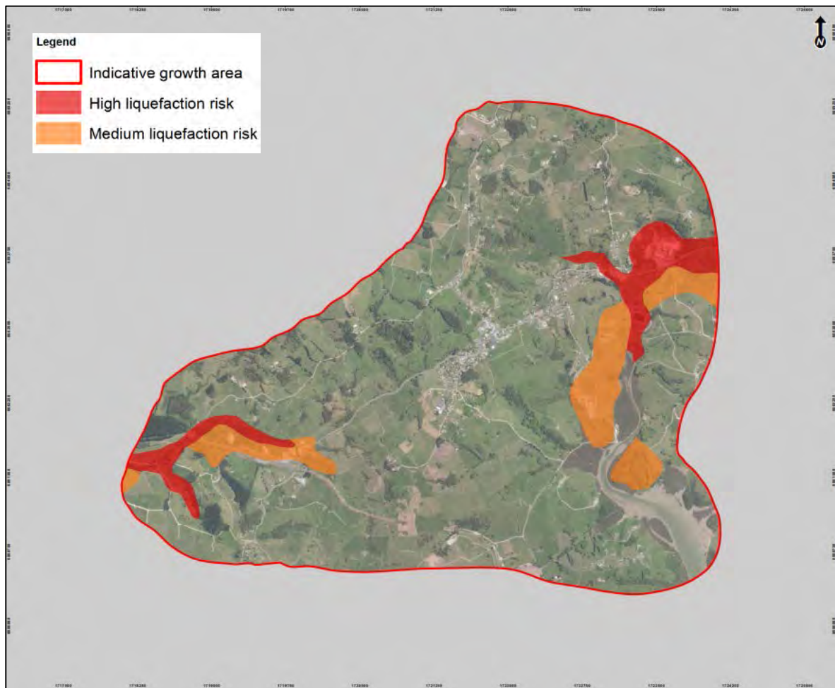
Figure 7: Liquefaction and Lateral Spread Susceptibility Plan
